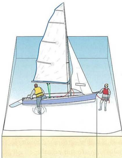
Helmsman boards and lowers the rudder and adjusts the centreboard
