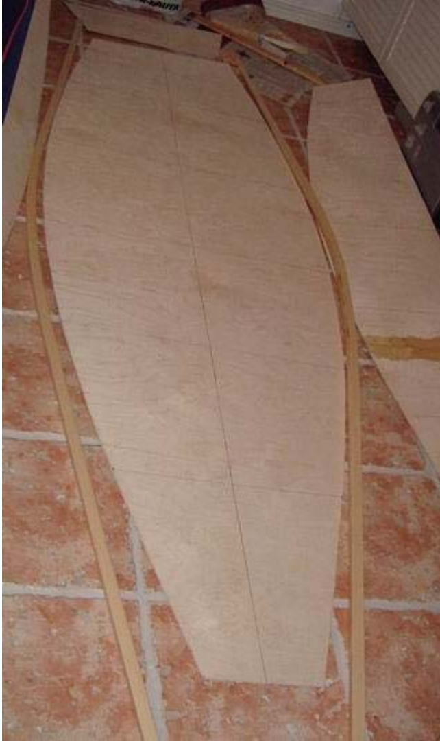
Sides butted with glass tape on either side of the ply and gunwale battens bent with the help of a heat blower gun.
