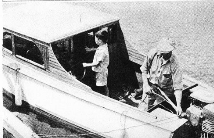
Trim appearance of Flight shows well in this aft view. She will do up to 30 m.p.h., depending on motor used. Note tumble-home, or inward sweep of sheer, at the stern
