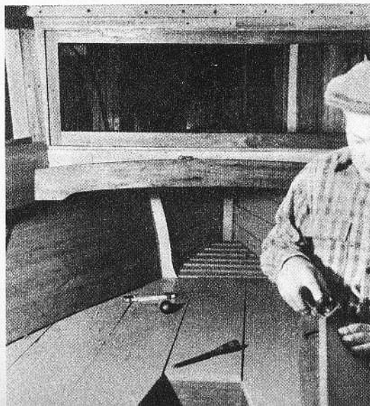
Left: Interior view of the half-completed cabin, showing windshield frame in place and berths in foreground. Below: Detail of frame. Notches for side and bottom battens are cut after frames have been set up.
