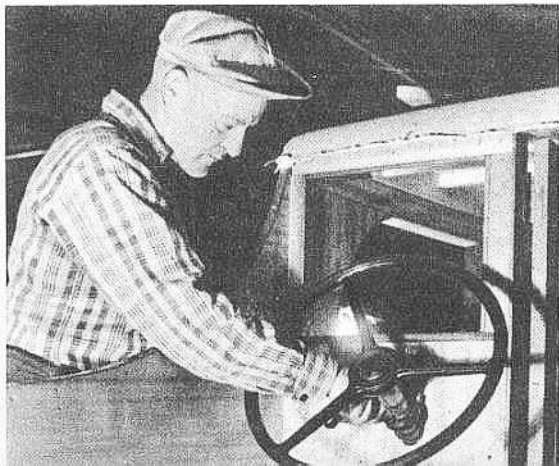
A Chevrolet steering wheel and post, with wood drum attached, are connected to the outboard motor by cable or rope.
