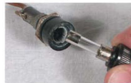
Panel fuse holder with glass fuse
