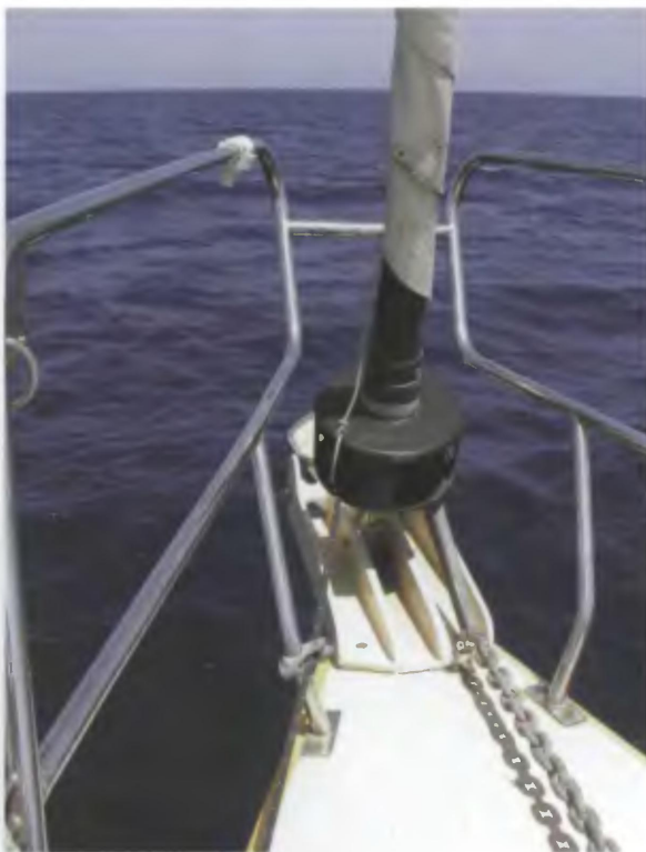
The loads on headsail roller reefing gears can be greatly reduced by running off the wind.
