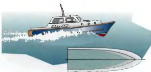
A semi-displacement hull
