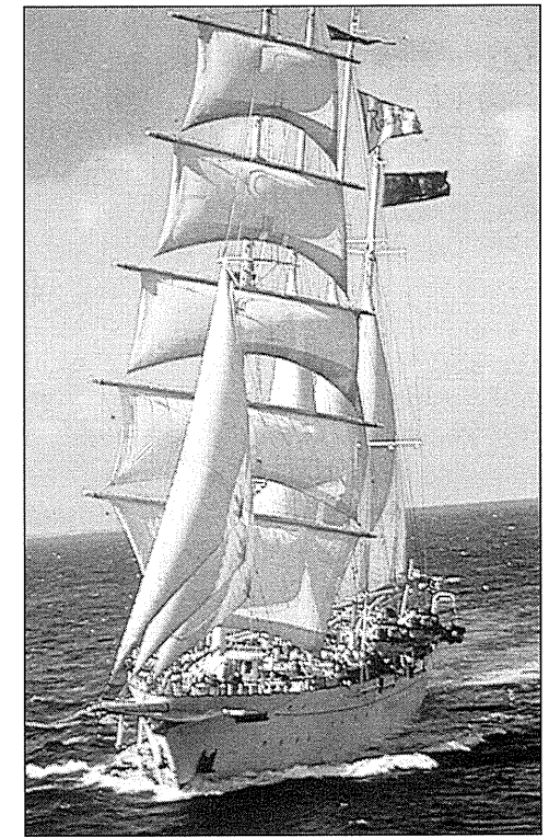
Fig 1.6 Star Clipper , a modern 3000-ton four-masted barquentine, built as a luxury cruise ship and carrying 170 passengers in air-conditioned cabins.
